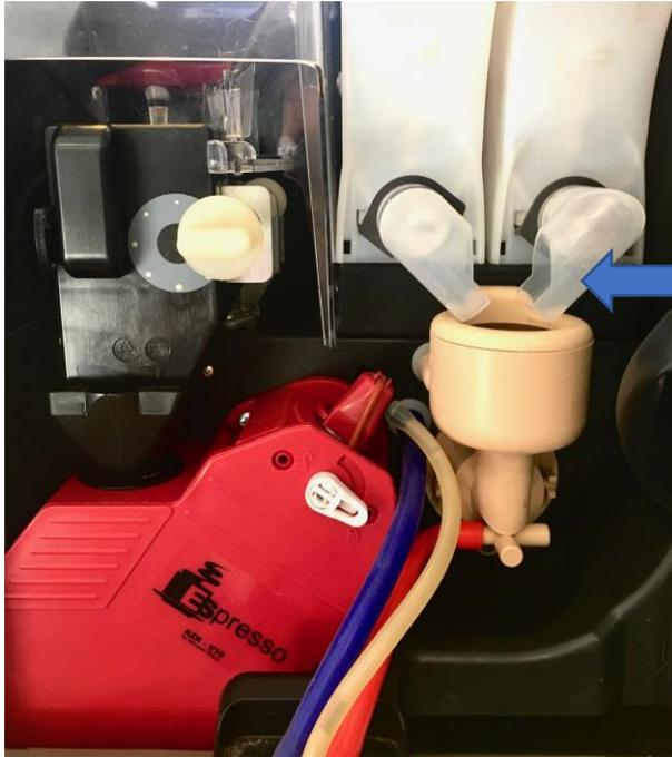
Ensure canister chutes are in the down position
