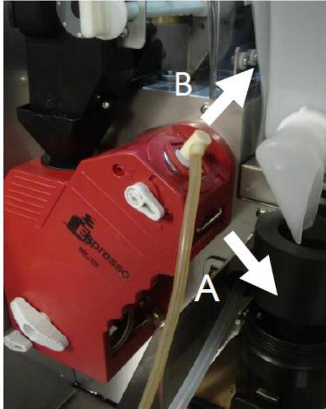
Remove the top piston from the brewer by pulling the lock (A) angled down away from the brewer. Once done, slide the piston (B) up out of the body of the brewer.
